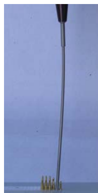
Incorrect use of tool. EXT tool may buckle.
