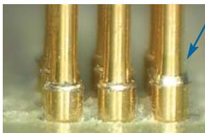
Diagram C: The shoulder of the termination pin has been damaged due to excessive hammering of the tool. Inconsistent set heights may also occur.
